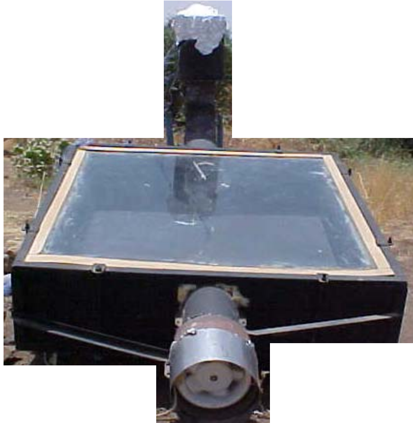
Plate 3.1. Forced convective solar dryer
