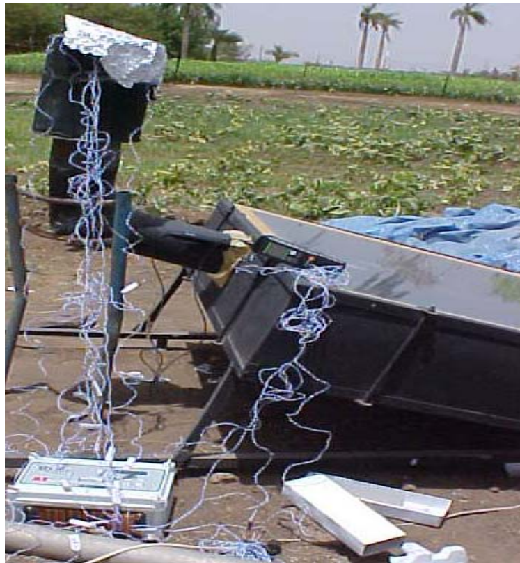
Plate 3.3 Delta T-logger sensors located at different places in solar dryer
