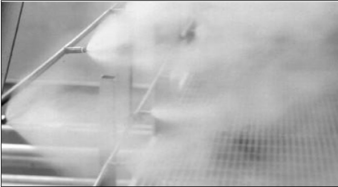
Fig. 4-7 Fogging system with high pressure impingement Nozzle [22]
